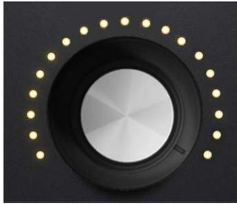
Press the “Wheel disable” button, and without releasing it, move the knob in the opposite sense to recover position. Having pressed the button “Wheel disable” the wheel does not turn on Titan One.
