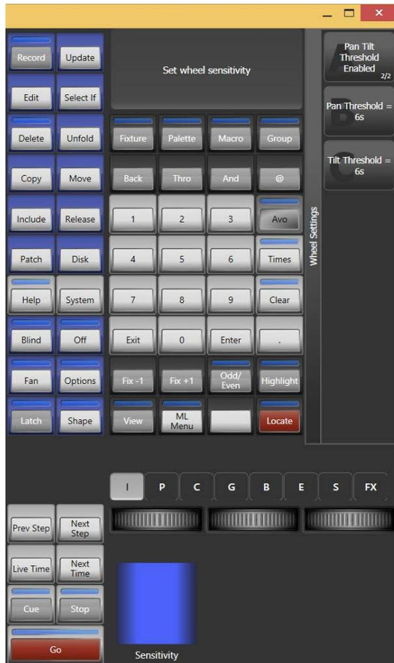
Don't forget to release the Avo button, as if it remains pressed wheels work always with very high sensitivity.
